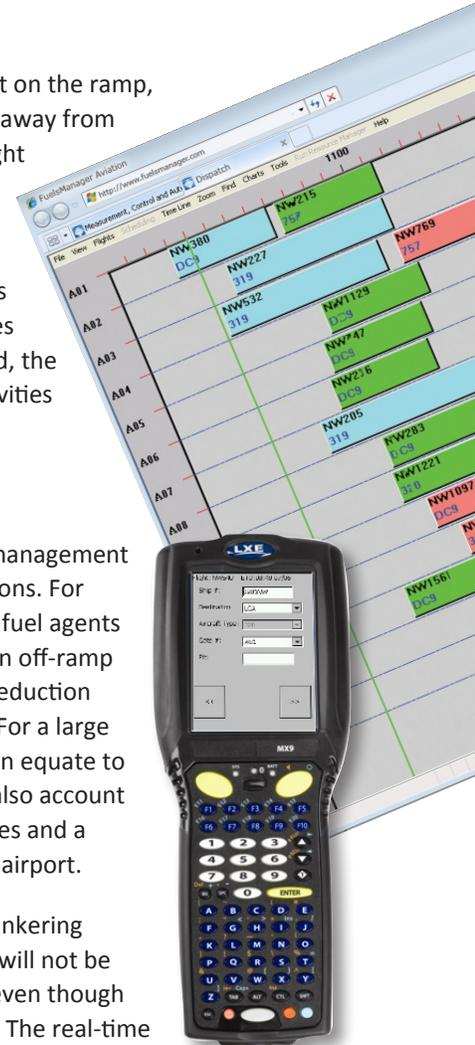
► *Dispatch assigns fuel requests to the Varec 9640 IntoPlane Handheld Computer. Fuel agents then use the handheld to record the aircraft fueling transactions.*
